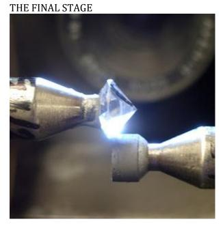
Here the remaining facets are polished and shaped to refract and reflect the optimal amount of white light. It is this stage that determines how much fire, brilliance and scintillation the diamond will have and as such it requires intense skill and experience. Here the ultimate goal is to obtain ideal proportions and perfect symmetry.
