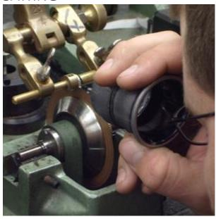
The marked rough diamond is then placed on a jewellers sawing spindle, where the blade is made from copper layered with a mixture of oil and diamond powder. The rough diamond is then lowered to the blade and cut where the marker has marked the stone.
