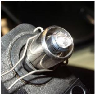
Here the rough diamond is set onto a 'dopstick' using a special type of cement to secure it in place. During this stage, two rough diamonds rub together and the friction wears the corners of the diamond down until it is round in shape.
